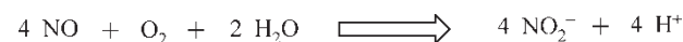
Scheme 2. Autoxidation of NO in aqueous phase in absence of biological material to nitrite.
